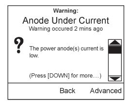
Faults: This is a safety related condition that has been detected by the heater.
